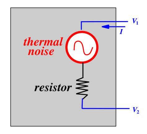
$$V_1 - V_2 - RI = V_{\text{noise}}$$
