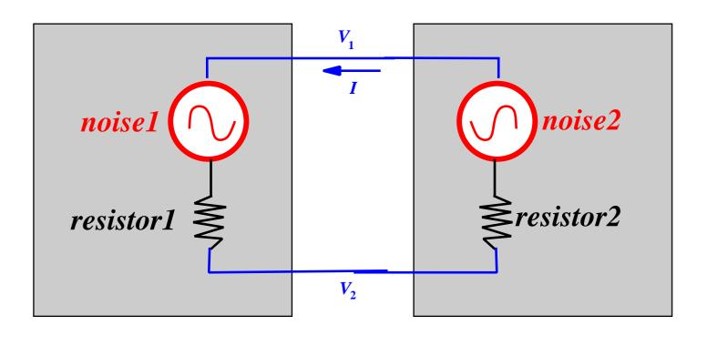
$$ightharpoonup I = rac{arepsilon_1 + arepsilon_2}{R_1 + R_2} \qquad V_1 - V_2 = rac{(R_1 + R_2)arepsilon_1 + R_1arepsilon_2}{R_1 + R_2}$$
