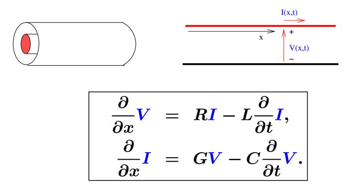
*R* the resistance, *L* the inductance, *C* the capacitance of the cable, *G* the conductance of the dielectric medium, all per unit length.
