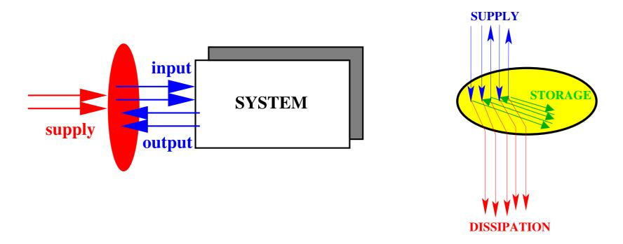
s(u, y) models something like the **power** delivered to the system when the input value is u and output value is y.
