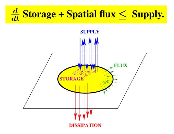
**Supply** = partly **stored** + partly **radiated** + partly **dissipated**.
