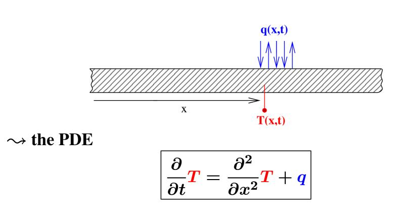
$(x \in \mathbb{R}, \text{ position}, t \in \mathbb{R}, \text{ time}), (2-D \text{ system})$ describes the evolution of the temperature T(x, t)and the heat q(x, T) supplied to / radiated away.
