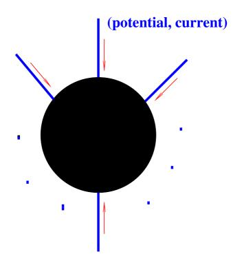
Dissipative w.r.t.  $\sum_{\ell=1}^{N} V_{\ell} I_{\ell}$  (electrical power).
