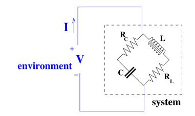
There are first order state repr. with an observable storage function.  $\Rightarrow$  can be synthesized with one capacitor, positive resistors, gyrators, and transformers.
