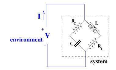
However, no reciprocal first order realizations (without gyrators) that use *only one* reactive element (a capacitor or an inductor), positive resistors, and transformers.
