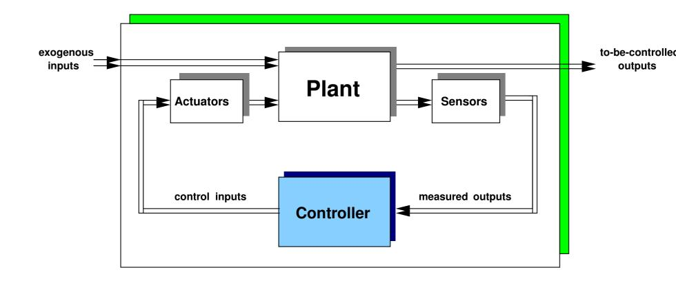
Plant, Controller, Cont'd system: i/o  $\cong$  signal processors
