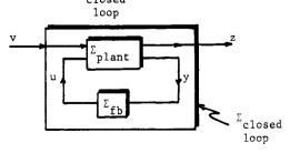
having v as input and z as output. A control system design problem consist in the question to design, for a given plant  $\Sigma_{plant}$  and a given design purpose, a feedback controller  $\Sigma_{feedback}$ such that the closed loop system  $\Sigma_{closed}$  meets the
