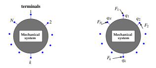
The *behavior* of the mechanical system is a subset  $\mathscr{B} \subseteq ((\mathbb{R}^{\bullet})^{2N})^{\mathbb{R}}$ ;  $(q,F) \in \mathscr{B}$  means that the position/force time-function  $(q,F)=(q_1,q_2,\ldots,q_N,F_1,F_2,\ldots,F_N):\mathbb{R}\to (\mathbb{R}^{\bullet})^N\times (\mathbb{R}^{\bullet})^N$  is compatible with the architecture and the element values of the mechanical system.
