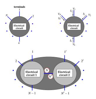
real variables, a potential and a current, at each terminal. The current is counted positive when it flows into the circuit. For the basic concepts of circuit theory, see [2], [6], or [1]. The setting developed in [?] and [6] has the same flavor as our approach.
