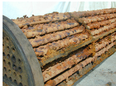
Fouling detection in heat exchangers
