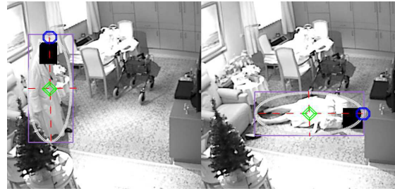
Fig. 4. Extraction of salient subject features used for fall detection. Purple rectangle: bounding box of subject; white fine segmented line: best-fitting ellipse within subject bounding box; double green diamond: center of mass; blue octagon: head position. (Small, filled black rectangle is not part of feature extraction set; it is inserted in the figure presentation here to maintain subject anonymity).
