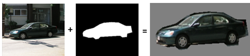
Fig. 6. An image of a car, plus its corresponding binary segmentation mask in a normalized bounding box.
