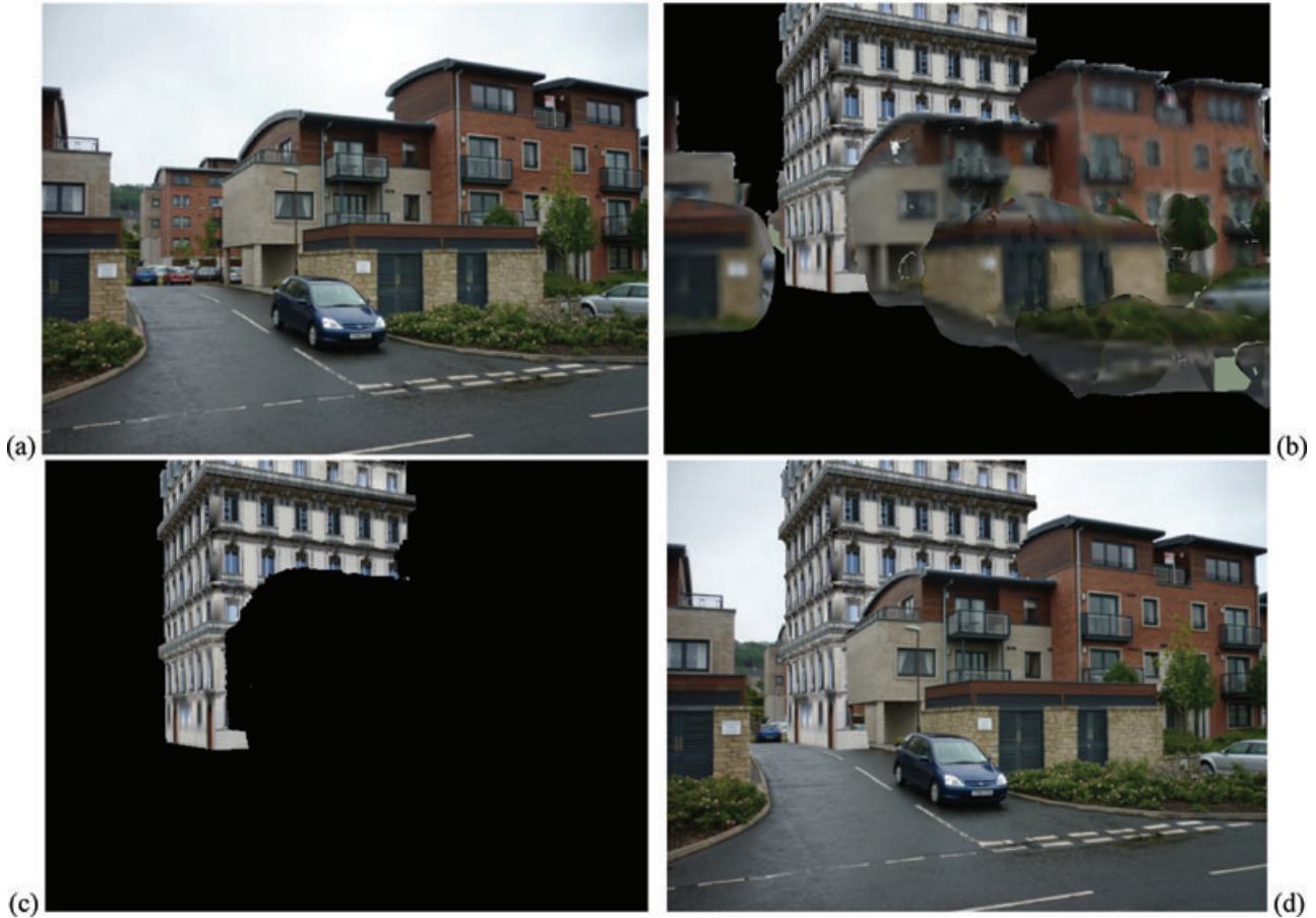
Fig. 6. The process to augment a target image: (a) target image; (b) virtual image obtained from the estimated pose and the target image’s internal parameters; (c) texture to be superimposed (overlaid) on the target image; and (d) augmented target image.
