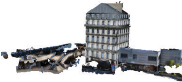
Fig. 4. Dense reconstruction of the EPFL campus scene obtained using ARC3D (Tingdahl and Van Gool, 2011). The scene is then augmented with a virtual Parisian-styled building.
