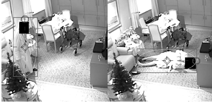
Figure 2: Extraction of fall features: full line: bounding box, fine dash line: bounding ellipse, diamond: center of gravity, octagon: head position (The black box is for privacy reasons)
