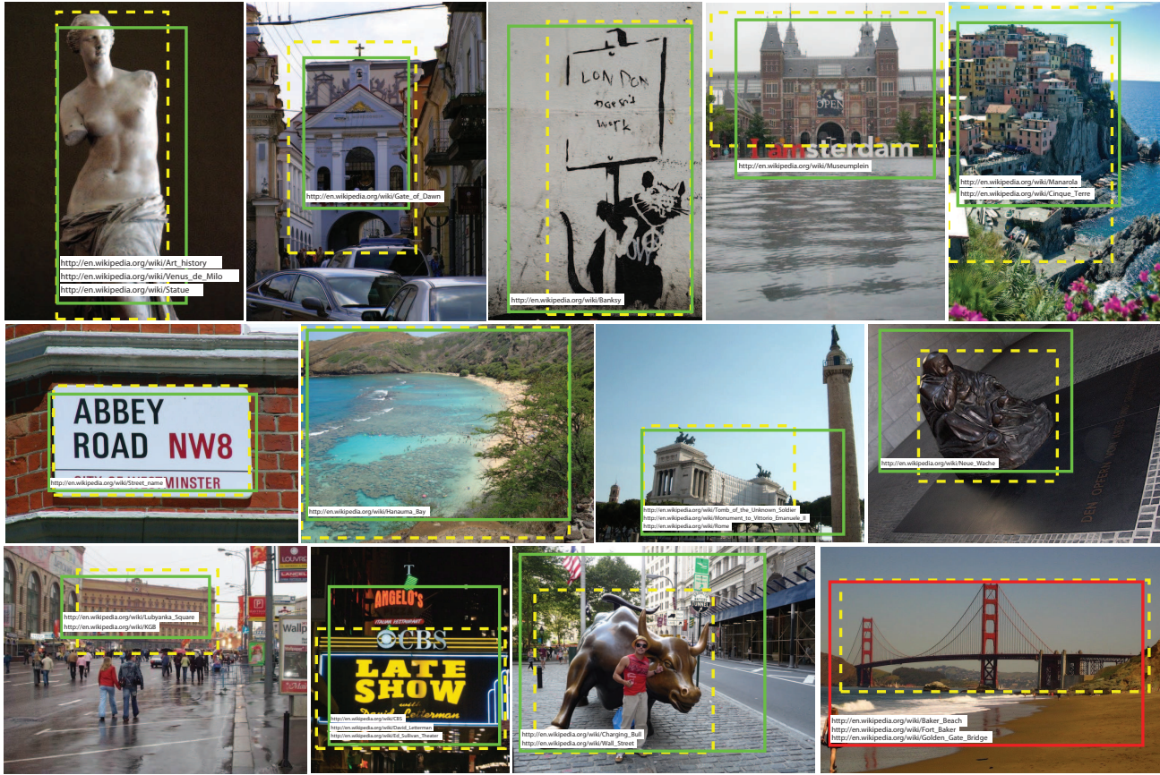
Figure 9. Results of automatic object-level annotation with bounding boxes. Groundtruth annotation is shown with dashed lines, correct detection with solid green lines, false detections with solid red lines. Auto-annotation with related Wikipedia articles is also shown. All results are also labeled with their GPS position and estimated tags (not shown here).
