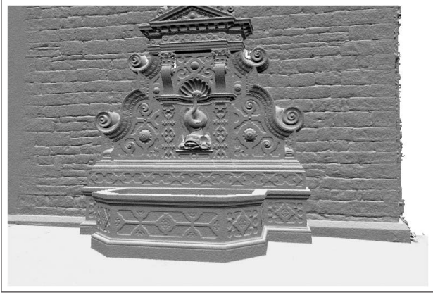
Figure 2. Diffuse rendering of the integrated LIDAR 3-D triangle mesh for the fountain-P11 data-set.
