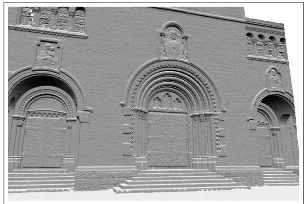
Figure 1. Diffuse rendering of the integrated LIDAR 3-D triangle mesh for the Herz-Jesu-P8 data-set.
