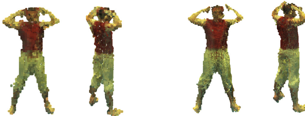
Fig. 3. The first two images show a reconstruction computed from five cameras at resolution 64^3 . The last two images show the same reconstruction at 128^3 resolution.
