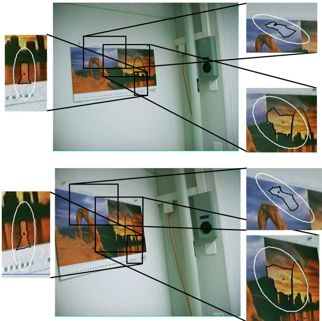
Figure 8. Affine invariant regions found with the intensity-based region extraction method and the linked points used to extract them.
