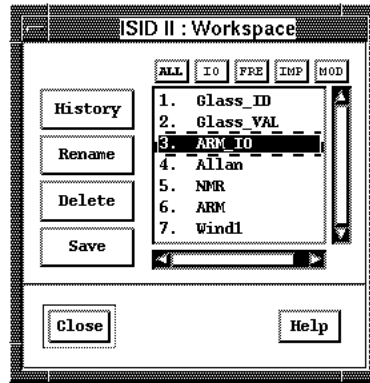
Figure 3.3 The ISID II workspace consists of a list of data objects. These data objects are loaded from user defined data. Alternatively they are outputs of algorithm blocks that were saved to the workspace. Through the data boxes, the objects in this list can be used as input to the chain. Recall that all of this can be done in an utmost elegant manner by just dragging and clicking with the three available mouse buttons.
