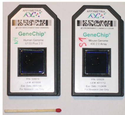
Figure 1.9: Example of an Affymetrix GeneChip. The GeneChip Human Genome U133 contains more than 54,000 probe sets and 1,300,000 distinct spots, covering the expression level of virtually all human genes.
