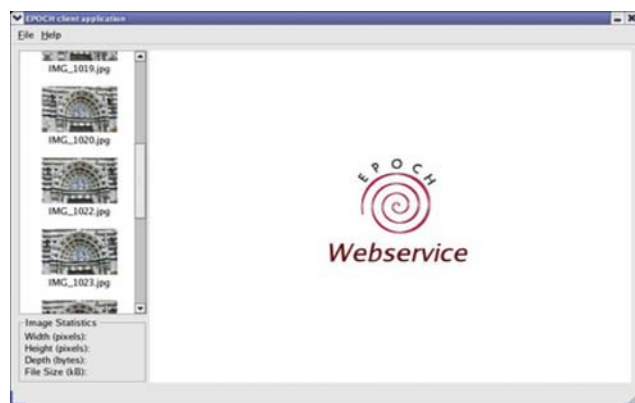
Fig. 3 Upload tool. Thumbnails of the images to be uploaded are shown as well as some statistics. When satisfied, the user uploads the images to the reconstruction server
