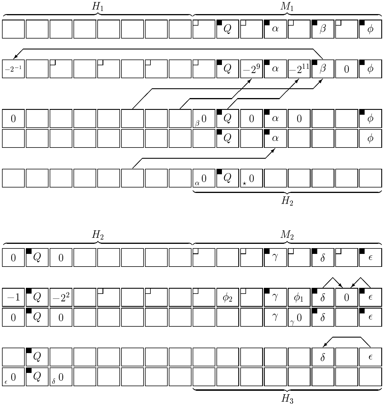
Figure 1: Schematic overview of the collisions of FFT-Hash. The state (e_0, \dots, e_{15}) is depicted before and after every step.
