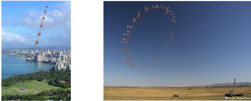
Fig. 4 An artistic vision with nearly vertical line (left, courtesy of TU Delft) and a real AWE system, with a lower elevation angle (right, courtesy Makani power, photo composite).
